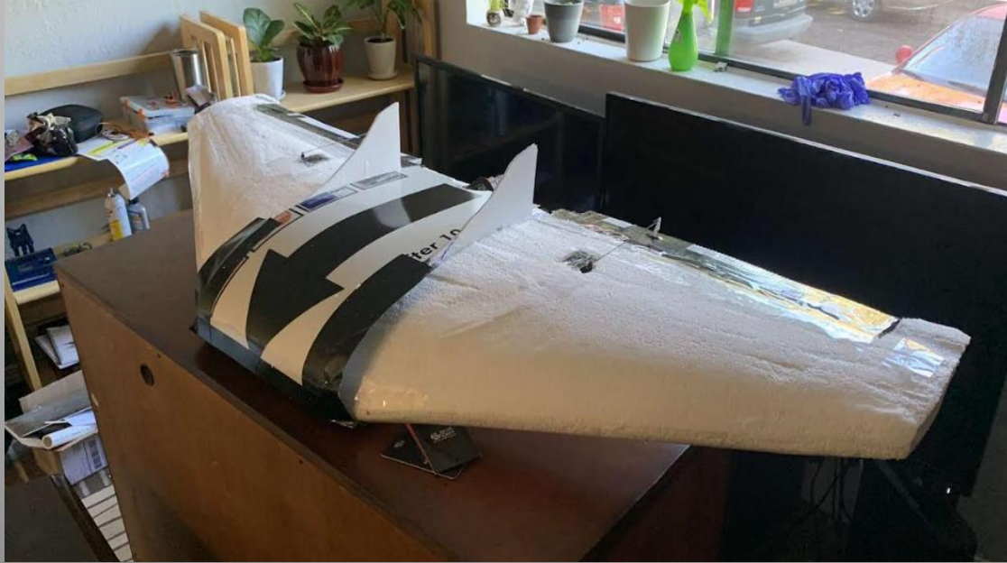
Prototype A: Hot Wire Foam Cut UAV w/ Motor System (No Solar)
