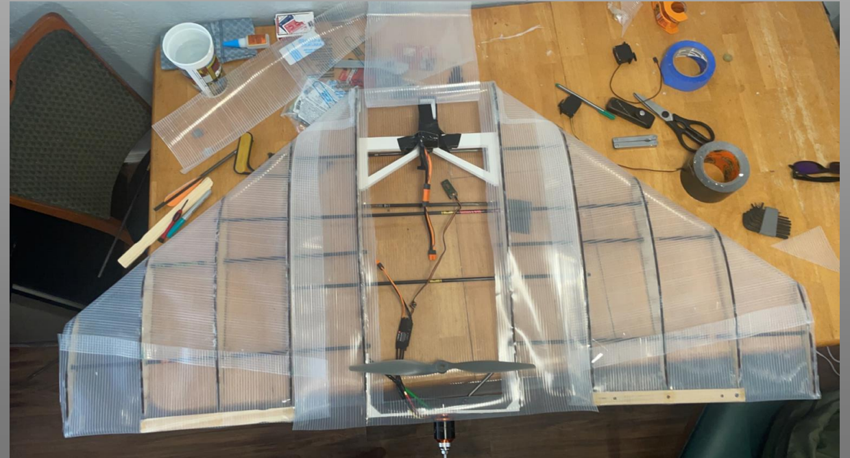
Prototype B: Wood Airfoil Cuts, Struts & Plastic Coating UAV w/ Motor System (No Solar)
